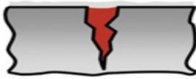
5 Application of developer
