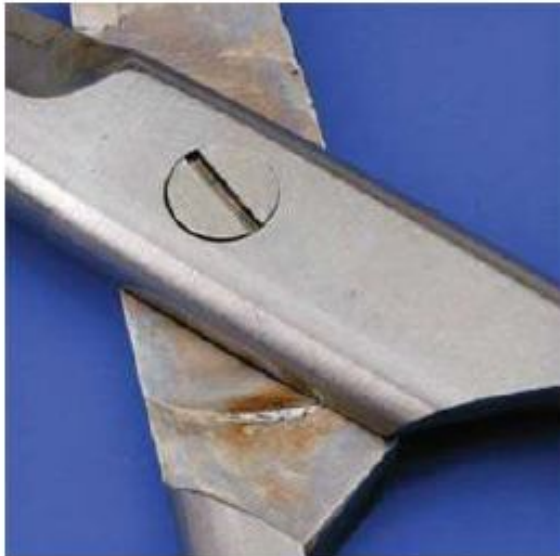
Example of Fretting Corrosion
