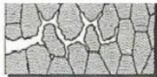
Intergranular fracture with microvoid coalescence
