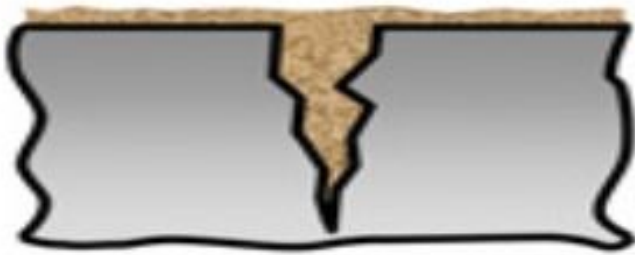
1 Crack filled with dirt
