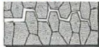
Intergranular fracture without microvoid coalescence
