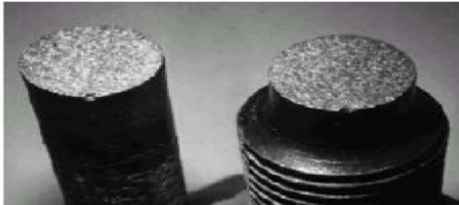
Brittle fracture in a mild steel
